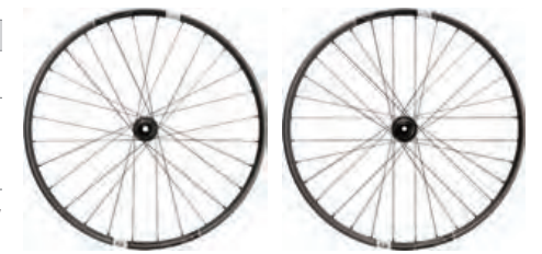
COMPLIANT FRONT WHEEL STIFF REAR WHEEL SPOKE COUNT: 28 INNER RIM WIDTH: 26.5 SPOKE COUNT: 32 INNER RIM WIDTH: 24.5
