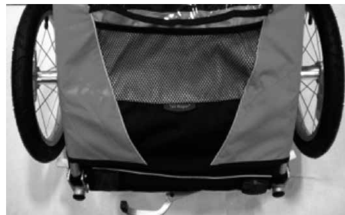
(写真 5) Tailgate fastened under cover
