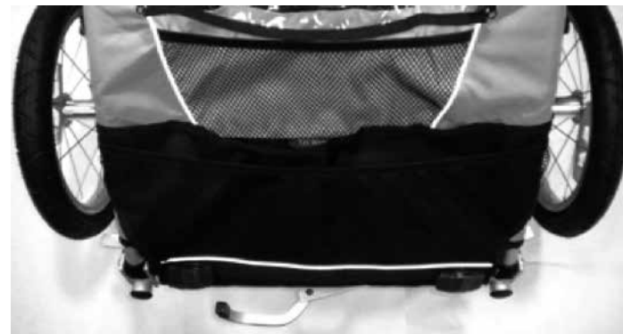
(写真 4) Tailgate fastened over cover
