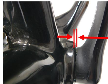
Note: The wave spring washer does not have to be completely compressed for proper use but does have to be in contact on both sides by the left arm and left bearing shield.
