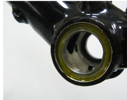
3. Apply a layer of grease on the outer edge of the bearing (3) to reduce friction between bearing and bearing shield, as well as improve protection from water and other contaminants.
